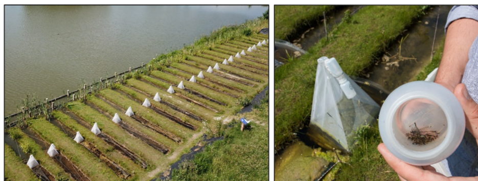
Fig. 1. Overview of the experimental site (Left). Shown are individual experimental ditches adjoining to a small lake. Each ditch was fitted with one emergence trap from which insects are caught and directly stored (Right).
